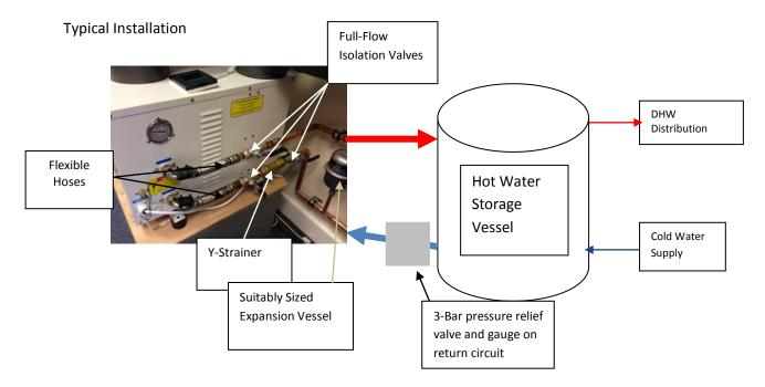
Please note that the expansion tank is not supplied as it depends on the configuration of the pipework and, therefore, the volume of that pipework and associated control fittings. However, an optional fitting kit is available from ESP, please ring for details or visit our web site.
