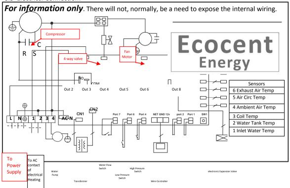
All electrical wiring MUST be carried out by a competent electrician and be in accordance with the latest I.E.E. Wiring Regulations. The Ecocent Energy is connected to the 13amp ring main via a 5A fused spur and the pre-installed power cord. It must be properly earthed.
