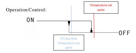
The Ecocent Energy will run until the temperature set point is reached. At that time, it will stop until the temperature of the stored DHW drops to more than 5°C below the set point at which point it will re-start.
