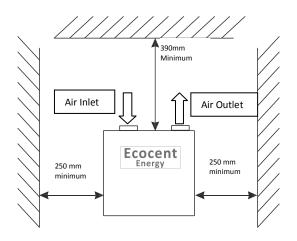
The unit must be sited out of direct sunlight and clear of areas of falling debris.
